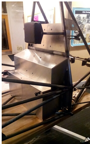
Figure 16: Photograph of the installed firewall's position in the car
