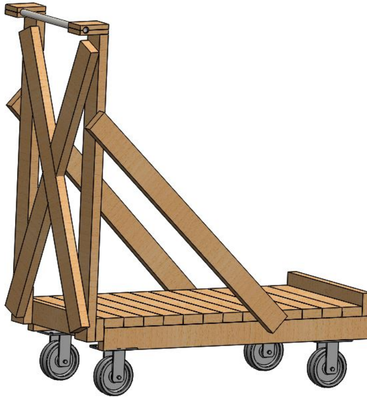
Figure 52: Cart with a deadman's lock for carrying the accumulator
