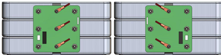
Figure 32: The location of the busbars, as seen on 2/4 segments.
