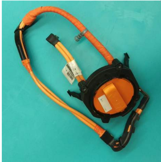
Figure 38: Manual Service Disconnect (Maintenance Plug)
